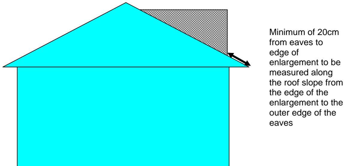
This 20cm set back will be required unless it can be demonstrated that this is not possible due to practical or structural considerations. One circumstance where it will not prove practical to maintain this 20cm distance will be where a dormer on a side extension of a house joins an existing, or proposed, dormer on the main roof of the house.
