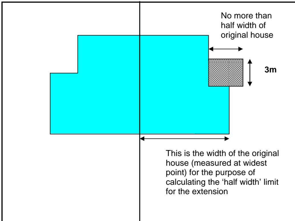
In the two examples above, the extensions would need to meet the relevant criteria for side and rear extensions i.e.:
